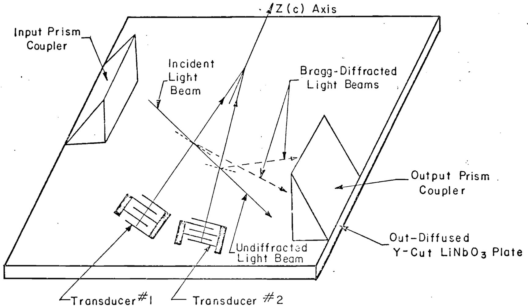
Figure 1. Guided-Wave Acoustooptic Bragg-Diffraction from Two Tilting Surface Acoustic Waves.
