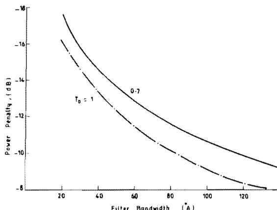
Figure 7. The dependence of the power reduction penalty on the filter bandwidth.
