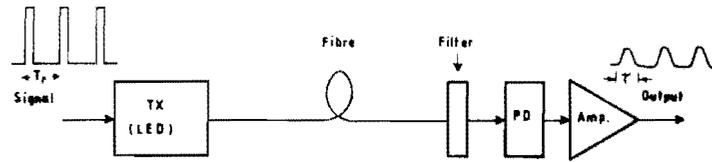
Figure 1. A block diagram of a digital fibre-optic communication link.
