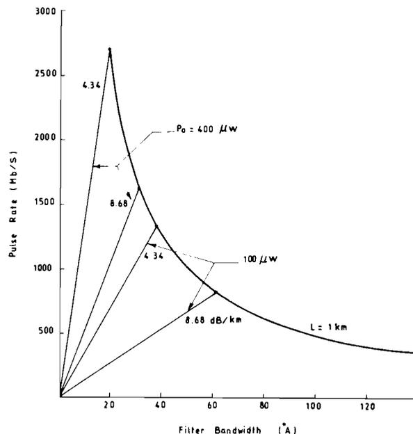
Figure 5. The dependence of the maximum information pulse rate on the filter bandwidth.  $L = 1$  km.
