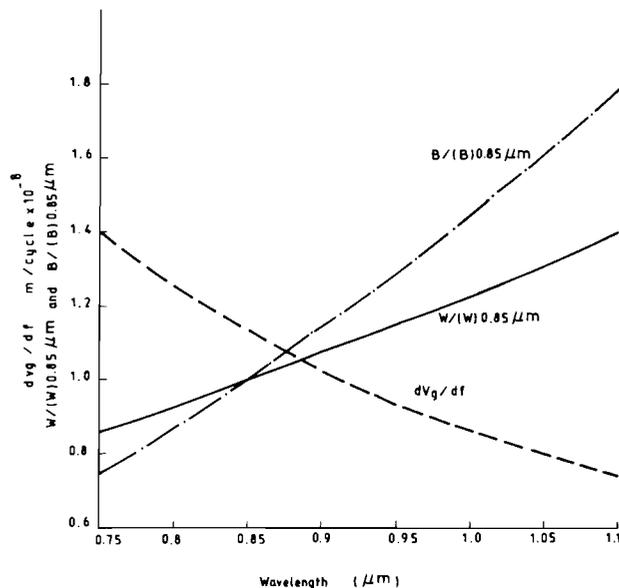
Figure 6. The dependence of the optimum filter bandwidth and the corresponding maximum information pulse rate on the central wavelength  $\lambda_0$  of the LED.
