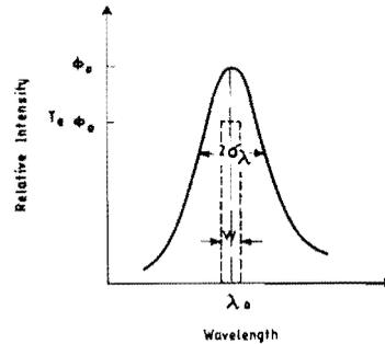
Figure 2. The transmission characteristics of the filter as compared with the spectral distribution of the output of an LED.
