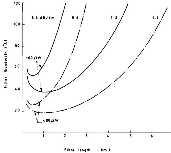
Figure 3. The optimum filter bandwidth to achieve maximum information pulse rate ( $\lambda = 0.85 \mu\text{m}$ ).
